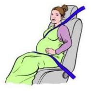
In this way the forces applied in a sudden impact can be absorbed by the body's frame.
